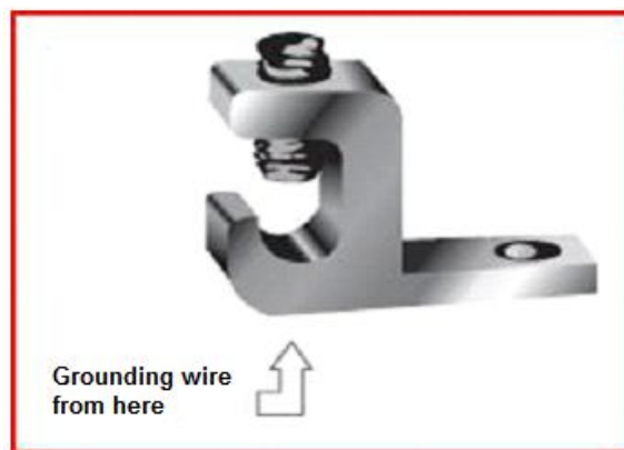
Figure 5 Schematic drawing for PV module grounding
